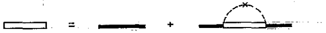
Figure 1. The Dyson equation for the one-electron Green function within the SCBA: solid and double lines represent the Green function of the free electron and the dressed one respectively; a cross is an impurity potential while a dashed line denotes the averaging over impurity positions.
